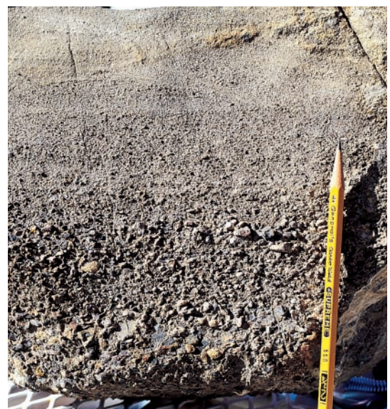
Figure 5.10 Graded bedding is produced by turbidity currents. It occurs in widespread layers, each layer generally less than a meter thick. Slumps off the deep continental slopes commonly produce great thicknesses of graded layers, which can easily be distinguished from sediment deposited in most other environments.
