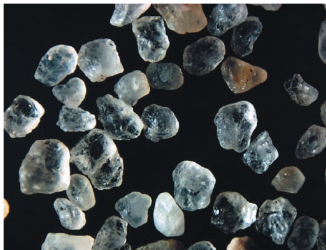
(B) A microscopic view of sand grains in sediment shows the effects of transportation by running water. The grains are rounded and sorted to approximately the same size.
